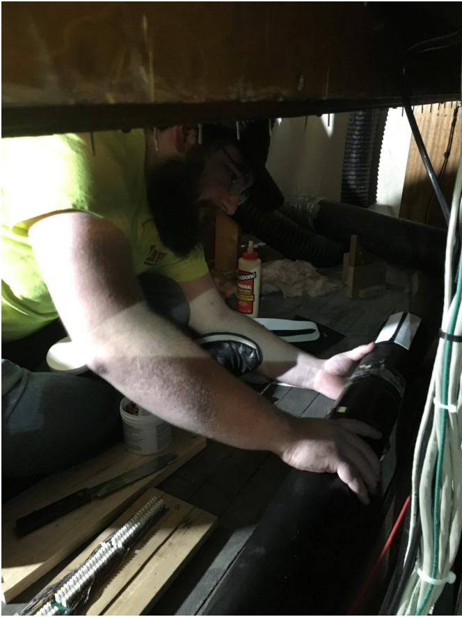
Pictured above, right and below: Technicians reinstall the refurbished bellows in the Great division.
