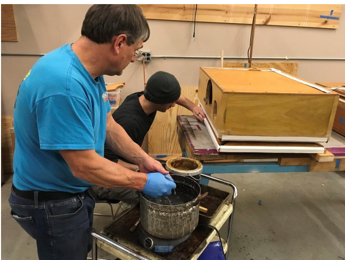
The old rubber cloth is removed from the Schwimmer bellows.
