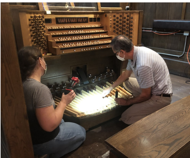
Trina Pirn and James Leek regulate the pedalboard's "touch" for Mr. Newman shortly before the concert. (All that fancy footwork needed a well-adjusted set of keys.) We are grateful for Leek Pipe Organ Company's exceptional care of our fine instrument.
